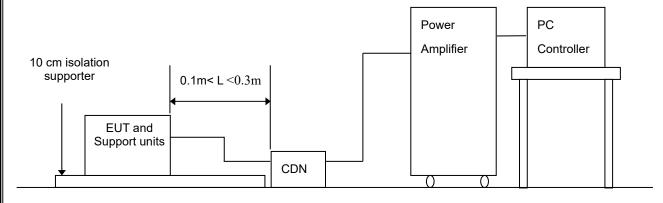
Note: 1. The EUT is setup 0.1m above Ground Reference Plane2. The CDNS and / or EM clamp used for real test depends on ports and cables configuration of EUT.
